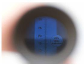
If the reading isn't what you expected or the borderline doesn't look as sharp as it normally does for that sample on an optical handheld refractometer, start again!
